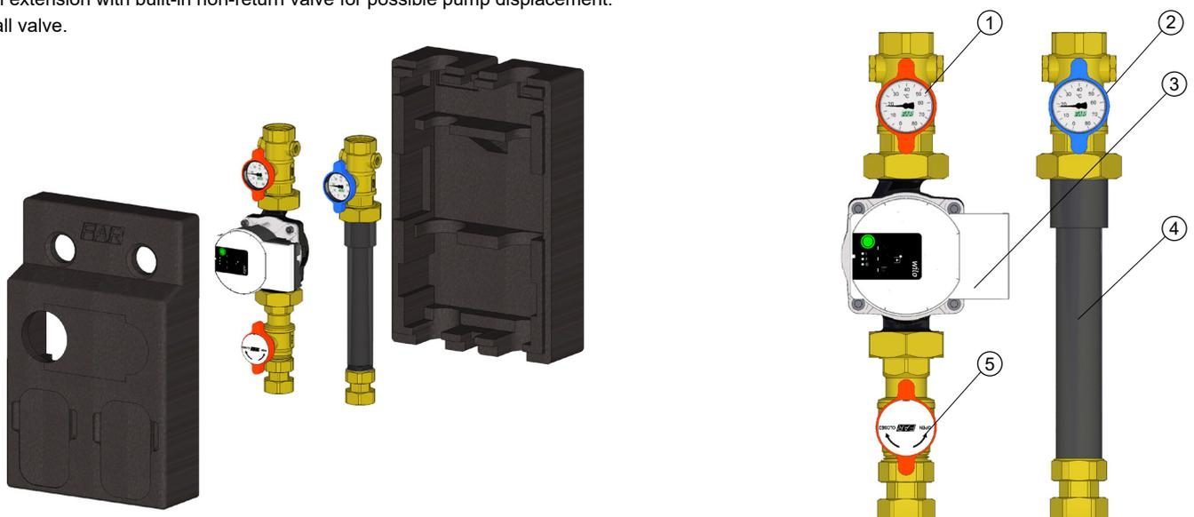
**FIXED POINT BOOSTER UNIT WITH THERMOSTATIC MIXER FOR LOW WATER TEMPERATURE SYSTEMS ART.2167**
